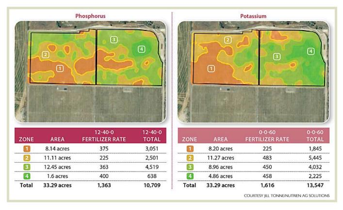
These maps show the variability in soils in an apple orchard for both phosphorus, at left, and potassium, at right, which are derived from scanning the block with a SoilOptix sensor and taking traditional samples for analysis. Nutrien agronomist Jill Tonne used these maps to set a variable-rate application plan to bring up the performance of weak spots in the block. Units are pounds per acre and total pounds.
