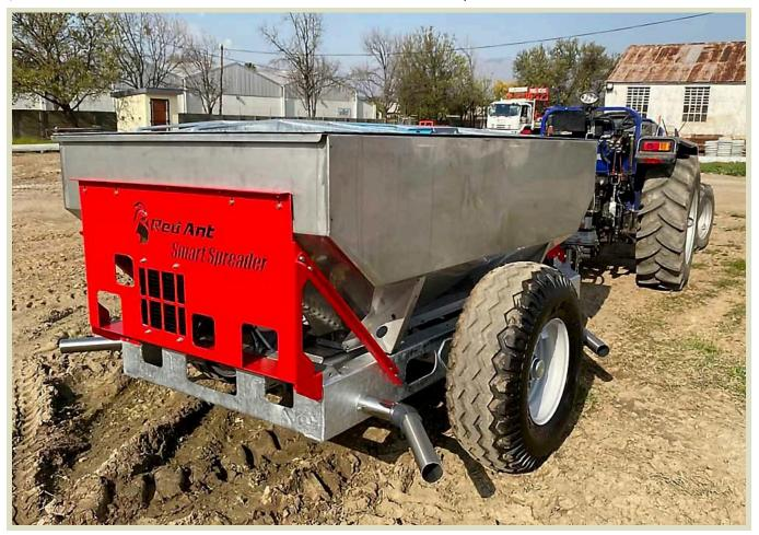
The Smart Spreader from Red Ant Agricultural Equipment of South Africa follows a task map to apply variable rates of fertilizer through an orchard. Red Ant designed this model specifically for the U.S. market, with a larger hopper and the ability to apply two products in one pass, to save on labor costs, according to engineer James Reid.
